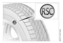
Run Flat tires are labeled on the sidewall with a circular symbol containing the letters RSC. Run Flat tires consist of self-supporting tires and special rims. The tire reinforcement ensures that the tire retains some residual safety in the event of pressure drop and driving remains possible to a restricted degree. The vehicle is equipped with Tire Pressure Monitor (TPM) or Flat Tire Monitor, which indicate a flat tire.
